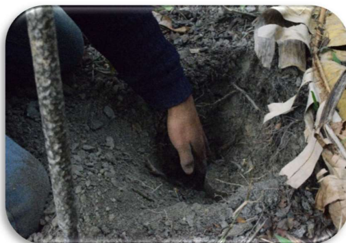
Collection of soil for Bulk density and Porosity using soil core sample
