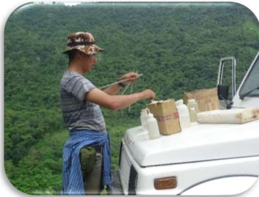
Preparation of water sample for DO and BOD
