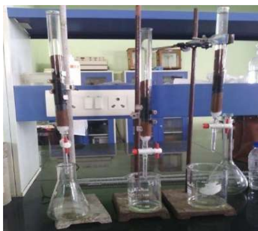
Fig.5.1. Set up of Sand supported column
