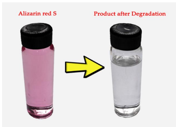
Figure 3.11 Snapshot showing aqueous deep red color ARS and the colorless end products obtained after degradation by \text{TiO}_2\text{-NP/PAC} nanocomposite
