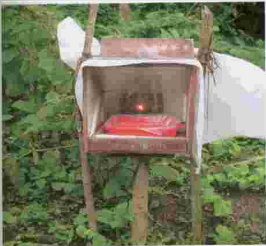
Plate IV (b). Light trap (Hurricane lamp type)
