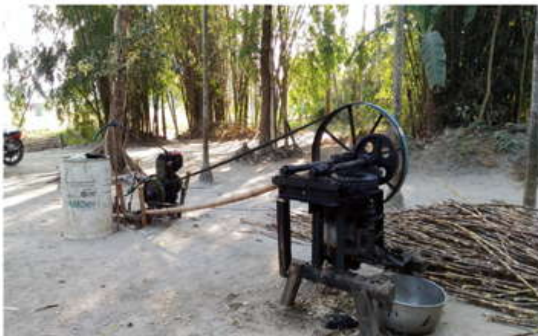
Plate 17: A home made machine to squeeze out juice from sugarcane.
