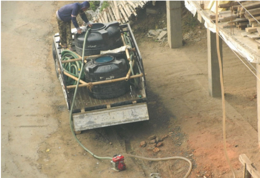
Fig 21: Water is delivered by using a petrol engine pump
