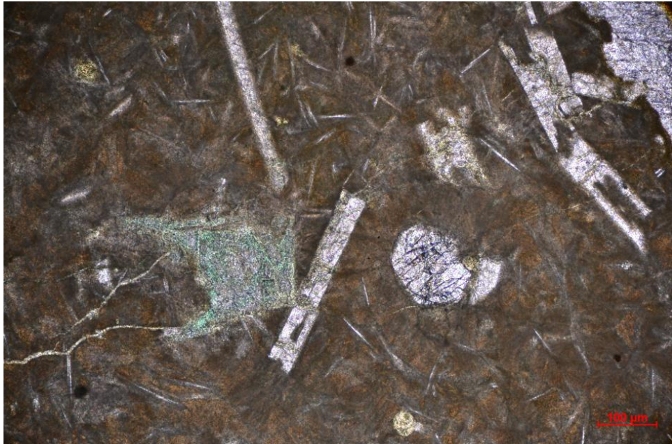
Plate 4.5: Phenocrysts of plagioclase, clinopyroxene and olivine in groundmass of acicular plagioclase microlites and dissolution of plagioclase to albite
