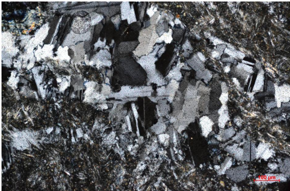
Plate 4.6: Plagioclase feldspar showing undulose extinction and swallow tailed twinning
