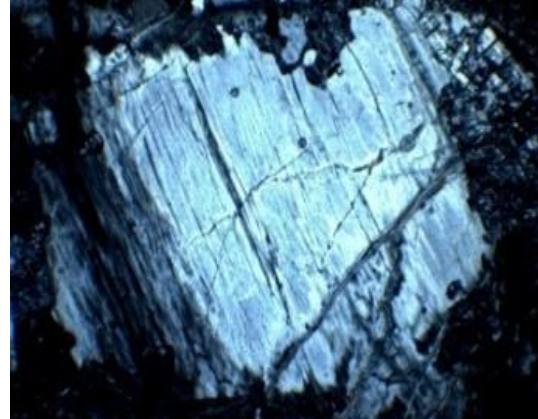
Fig. 3.1.9: Xenoblastic orthopyroxene showing Corrosive structure at outer margin (width of photo is 4mm, cross polar).
