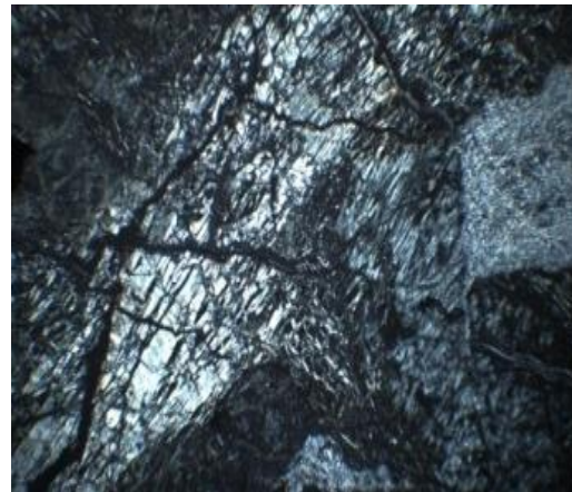
Fig. 3.1.11: Growth of serpentine into asbestiform chrysotile (width of photo is 4mm) in extremely serpentinised ultramafic (cross polar).
