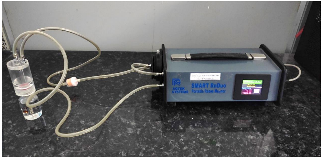
Fig. 2.12: Set up for measurement of ^{222}\text{Rn} in water.
