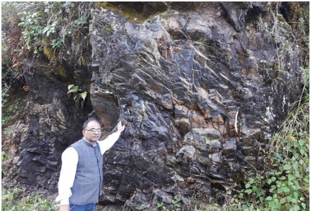
Figure 2: Field Photograph of Phokpur magnetite deposit along road cutting showing its jointed and compact nature.
