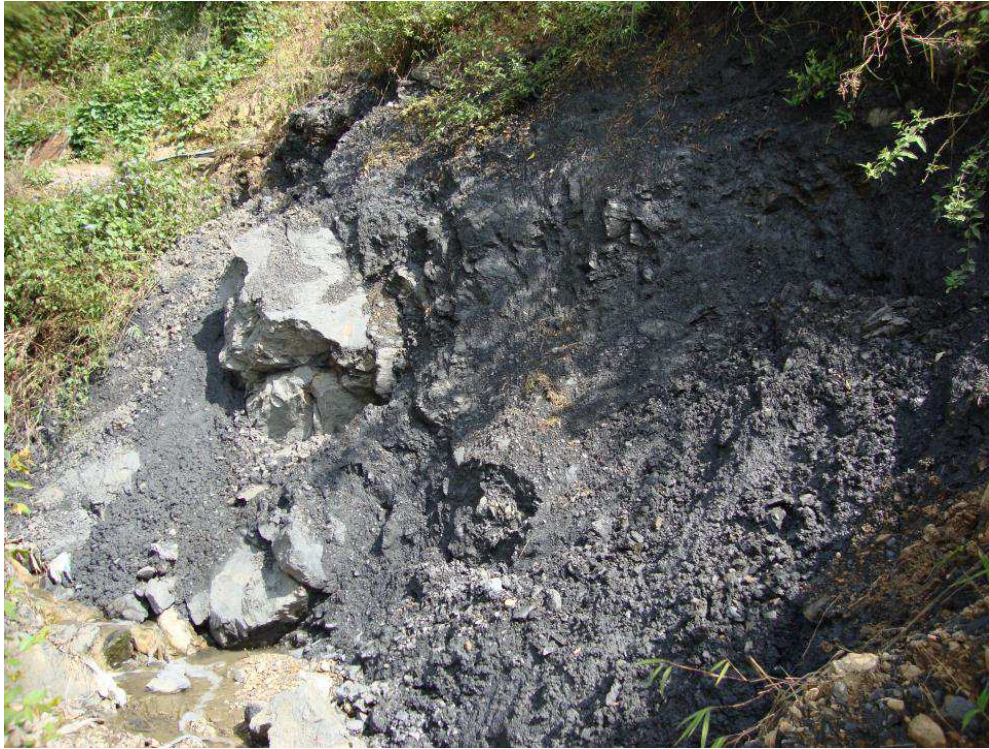
Plate 5: Disang shales exposed along nallah section at Midland colony (plastic and expansive)
