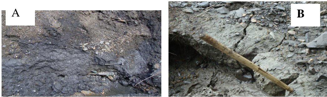
Plate 7: Swelling and expansion of highly plastic shale/clay at (A) Naga Hospital slide and (B) Dzuchie (KMC garbage Dumping site) slide
