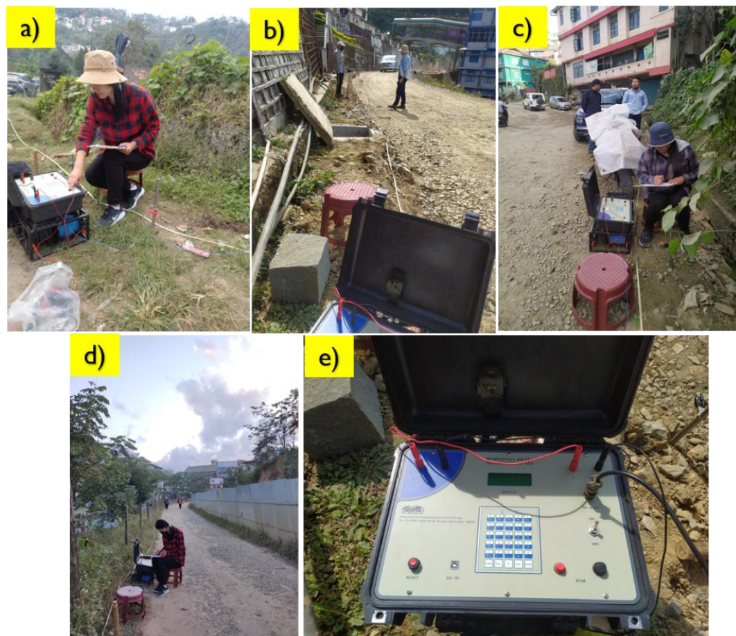
Fig. 3.2: a) Taking VES 1 data at Forest colony b) Measuring the length of spacing for current electrodes from VES 2 at Cathedral c) Noting the resistivity data from VES 4 data at Kenuozou colony d) Measuring the resistivity data from VES 5 at High School colony
