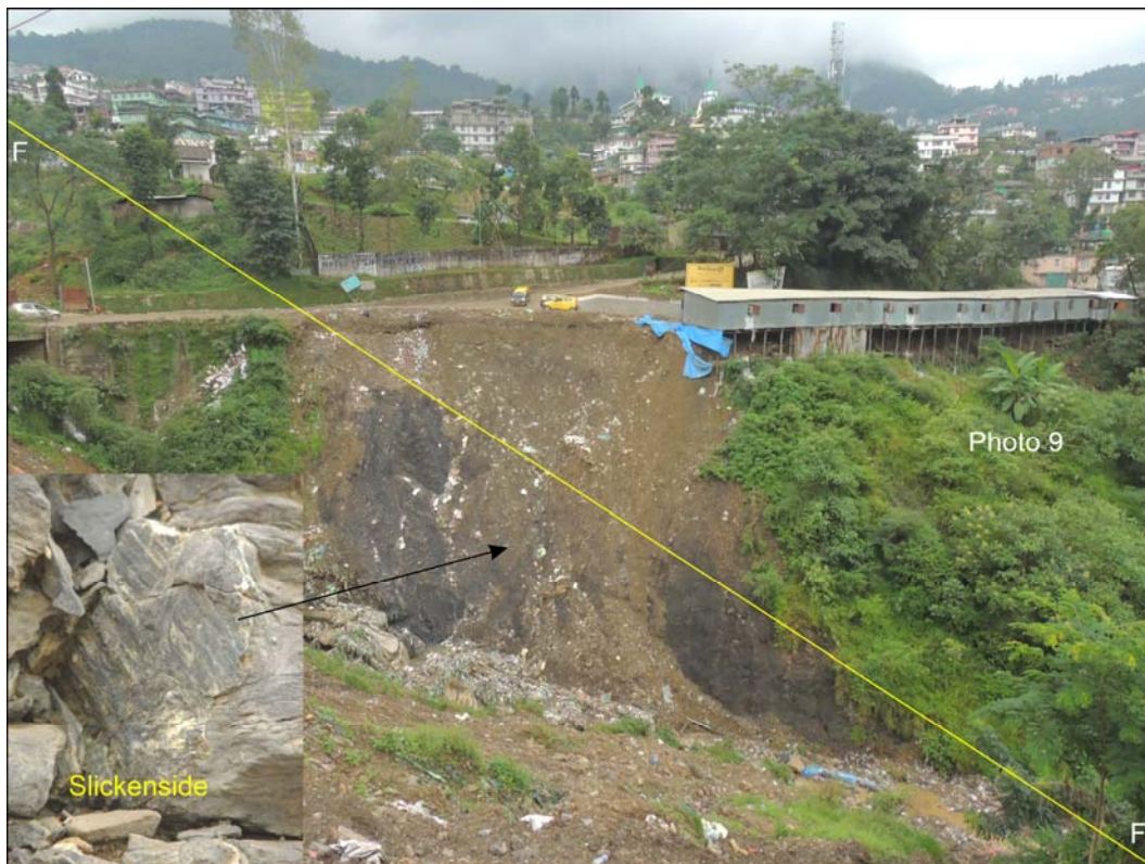
Fig. 4.1.15: Field photograph showing condition of slope due to strike-slip fault (Inset: Slickenside on western bank of river)
