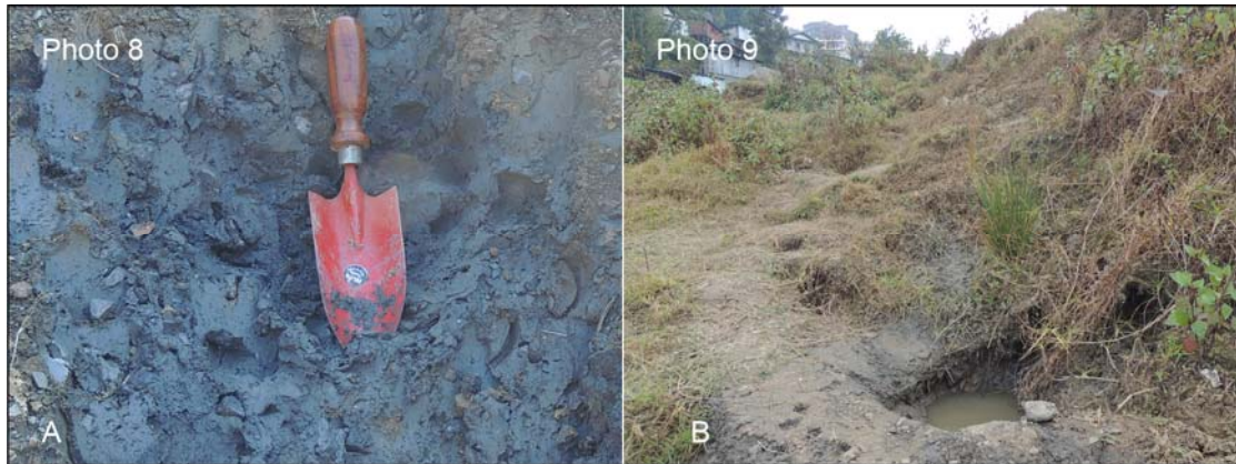
Fig. 4.2.14: A - Slope material constituting clay deposits; B - Water seepages observed during dry season
