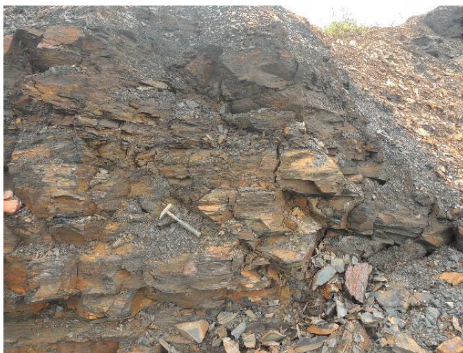
Fig. 6.1.5: Shale outcrop with large open fractures at Pezielietsie slide zone (2018)
