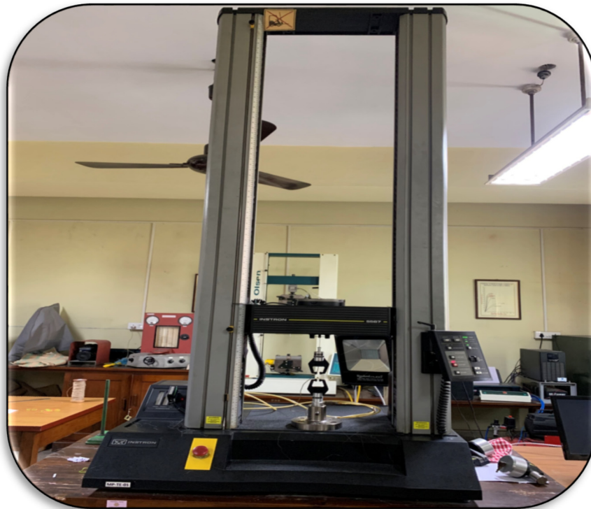
Plate 4: Measurement of individual fibre length to determine fineness and Universal Testing Machine for assessing tensile properties
