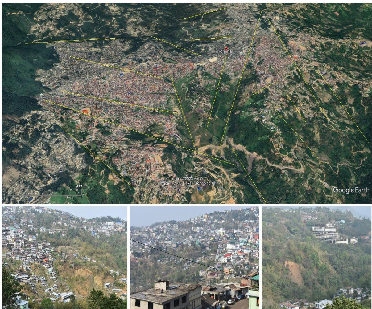
Plate 3.1: Aerial view of Kohima city showing unplanned urbanization over steep unstable slope along tectonically active lineaments (Above) as evident by number of landslides, debris fall, creeping, land subsidence events continually taking place in such zones (Lower left and right images).
