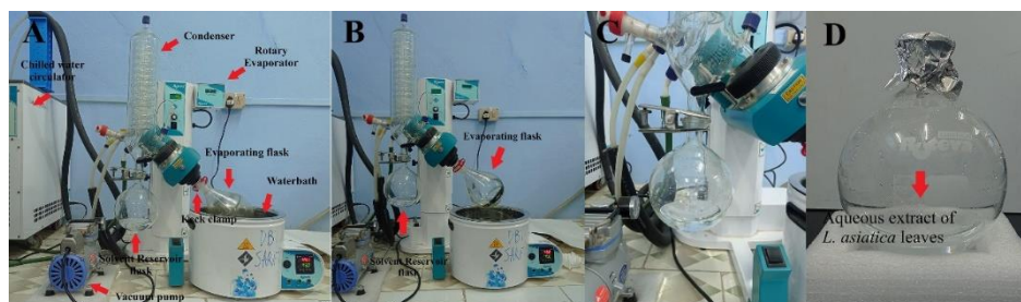
Figure 2.6. Running a rotary evaporator system with secured functioning components and storing the aqueous extract in the receiving flask/solvent reservoir .
