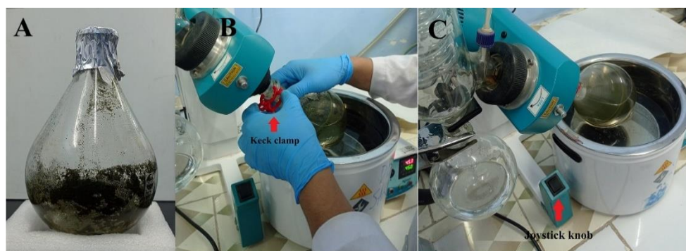
Figure 2.2. Storing solution in the evaporating flask and securing it with the Keck clamp and joystick knob . Solution stored in the evaporating flask (A) and secured with
