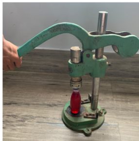
Step 8: Filling hot into sterilized bottles and corking
