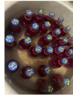
Step 9: Pasteurization (80°C for 10 mins)
