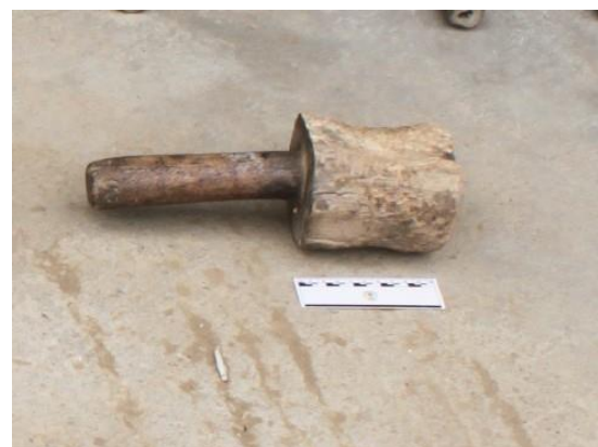
Plate 7: Types of wooden mallet ( Tshüzhie ) - one type is used for hammering big logs, while the other is used for bamboo crafts and handicraft works, demonstrating functional variations in Indigenous tools
