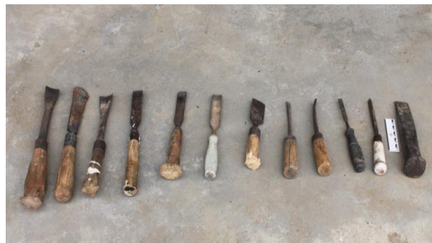
Plate 10: Assorted types of mini chisels used for intricate wood carving and detailed craftsmanship in traditional architecture and handicrafts, reflecting indigenous knowledge of specialized tools and techniques.
