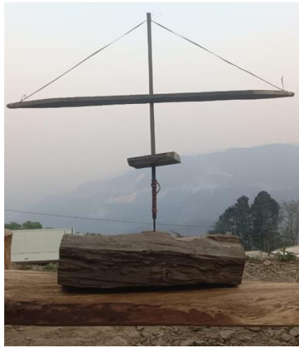
Plate 11: The Indigenous hand drill, a vital traditional tool used in architectural construction, valued for its cultural significance and practical function ( Photo courtesy: Neitshope Lasuh )
