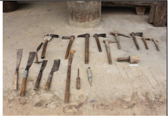
Plate 9: Types of Axe, dao, mini wooden mallet, and chisels – traditional tools used in domestic architecture.
