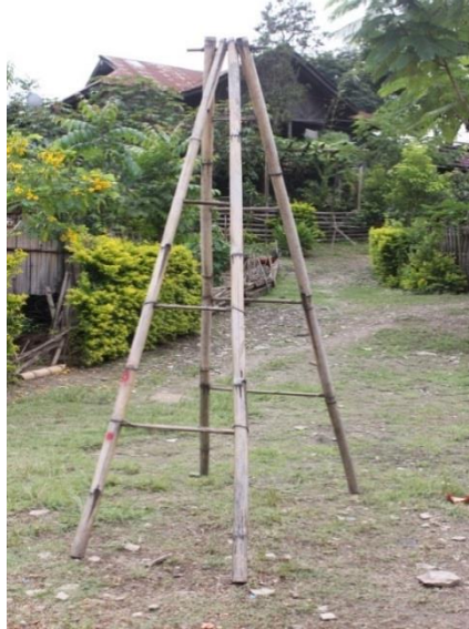
Plate 16: Triangular bamboo ladder – an innovative indigenous structure designed to provide stable and balanced access during domestic construction, demonstrating traditional engineering solutions tailored to vernacular architectural needs.
