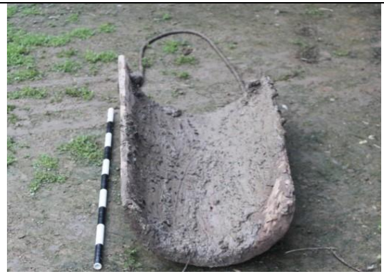
Plate 13: Nyosü – a traditional earth-moving tool used for hauling mud, leveling ground, and collecting large stones.
