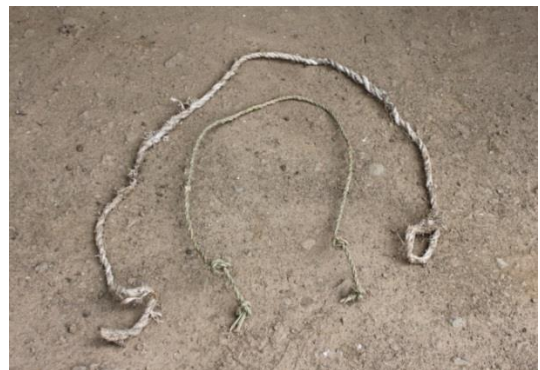
Plate 17: The measurement twine or string ( Khapvo rho ) is traditionally used to measure and secure bundles of Imperata cylindrica (thatch) in Naga construction. (Measures 6 feet 5 inches and 5 feet 2 inches)
