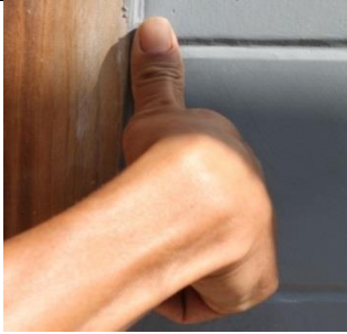
Plate 18: Inch ( Puthe ), traditional measurement technique using the thumb for marking dimensions in woodwork
