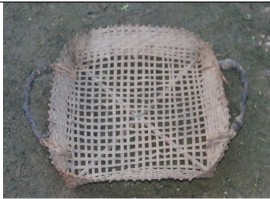
Plate 12: Nyopvo – Indigenous bamboo basket engineered for efficiently carrying mud during house construction
