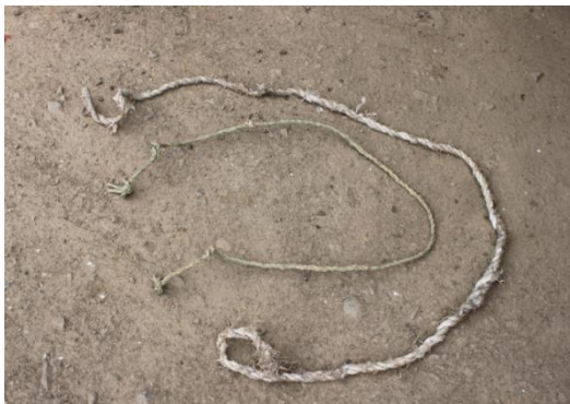
Plate 17: The measurement twine or string ( Khapvo rho ) is traditionally used to measure and secure bundles of Imperata cylindrica (thatch) in Naga construction. (Measures 6 feet 5 inches and 5 feet 2 inches)
