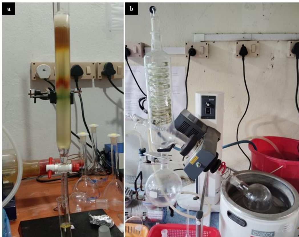
Figure 15. (a) Purification of partially purified BS through column chromatography and (b) Recovery of purified fraction of BS through a rotary evaporator system
