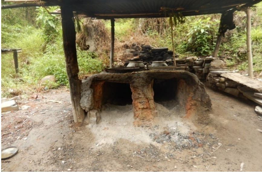
Plate No. 6. Peletkie Salt Kitchen with double fire hearth
