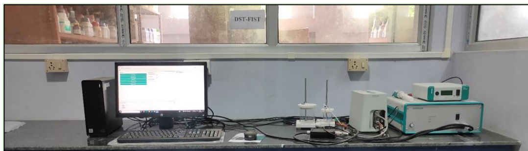
Figure 2.13. PGSTAT 204 and Nova 2.1.8 loaded on computer.
