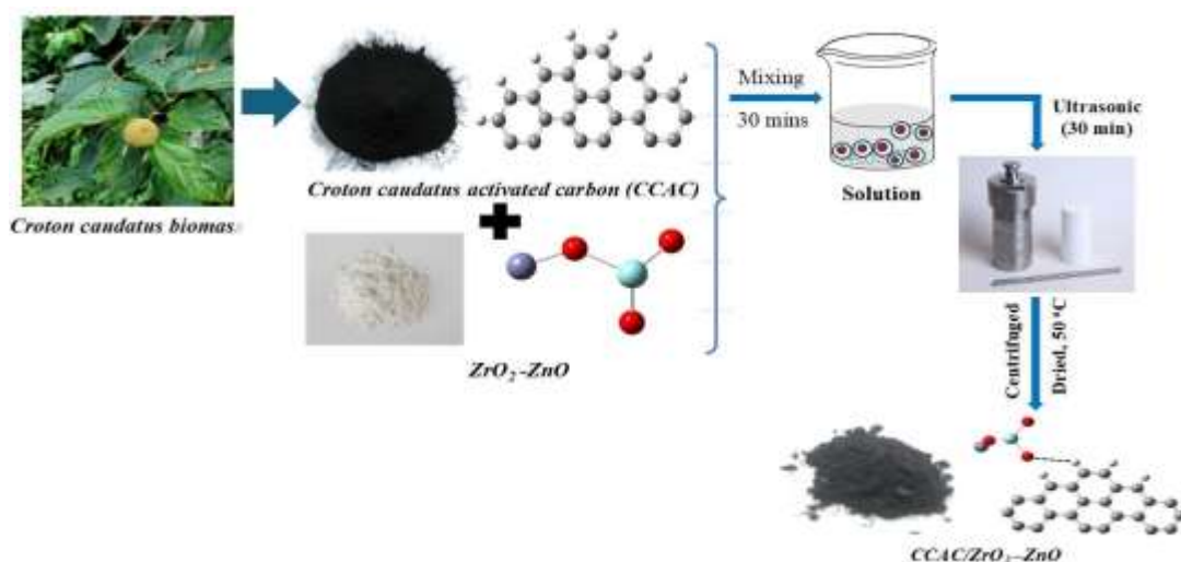
Scheme 5.1. Schematic illustration of the synthesis procedure for CCAC/ \text{ZrO}_2\text{-ZnO} nanocomposite.
