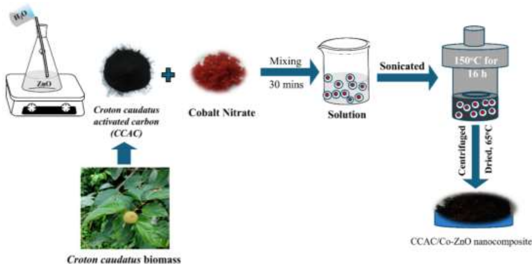
Figure 6.1. Scheme for preparation of the Croton caudatus activated carbon (CCAC)/Co-ZnO photocatalyst.
